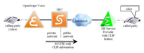
Figure 10 Example: CLIP Information Exchange (Outgoing Call to Service Provider)
